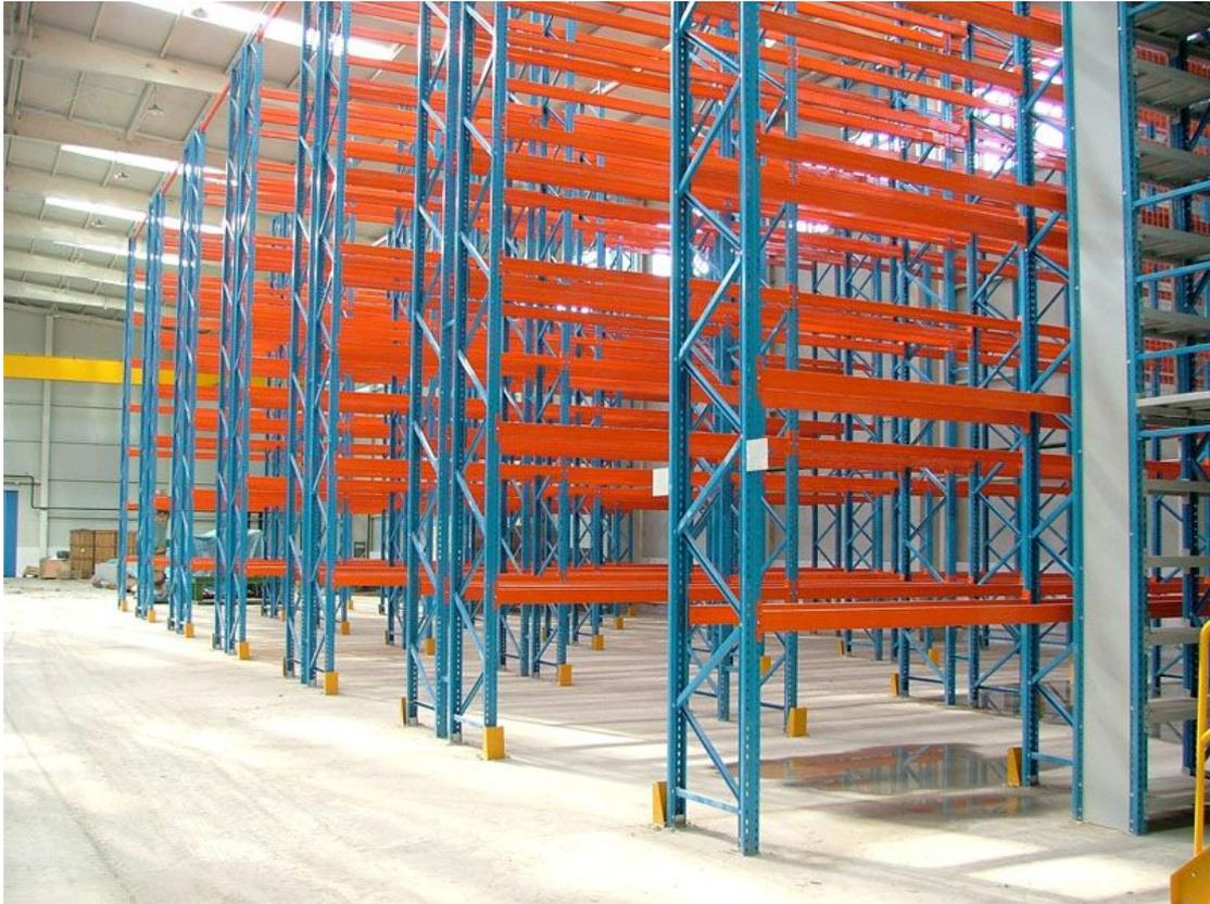
**Pallet Racking** is a special storage system to conserve cargo put on pallet. Each pallet need one position, thus it's also called pallet position racking. The cargo is 100% selective, thus it's also named selective pallet racking. The major components of racking system is upright frame and beam. Pallet Racking system is simple but reliable. According to the warehouse turnout situation and loading capacity, there are various of specification and size to be chosen.
